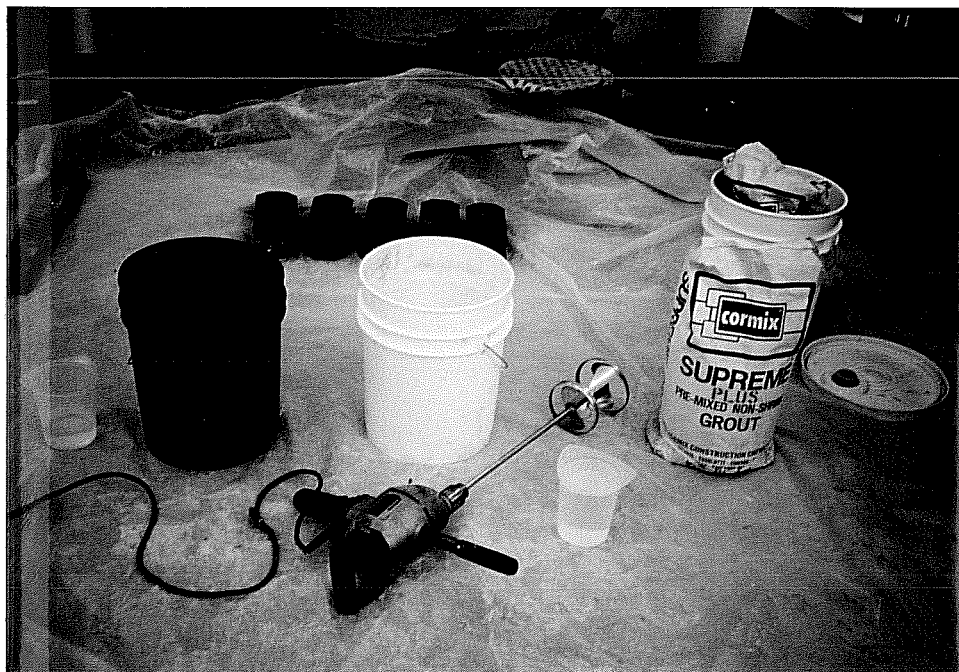
Figure 3.10 Grout Mix Set-up
